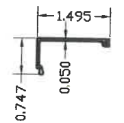
9 DOOR SCREW COVER 6063-T6 ALLOY
